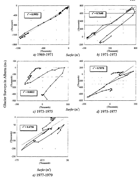
Figure 4.11: Scattergrams showing the relationship between Haumann calculations of volumetric change using DEMs and from Glacier Surveys in Alberta. Measurements from successive elevation zones connected by lines. This shows that often several different linear relationships exist in the data set of each interval.
