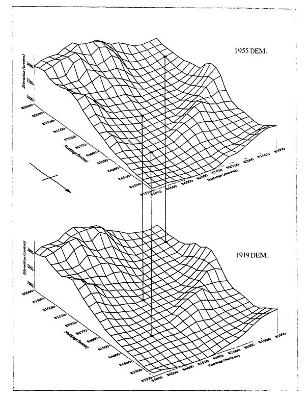
Figure 3.17: Calculation of surface change. Identical nodes are selected on two DEMs and the vertical difference between the values is calculated.
