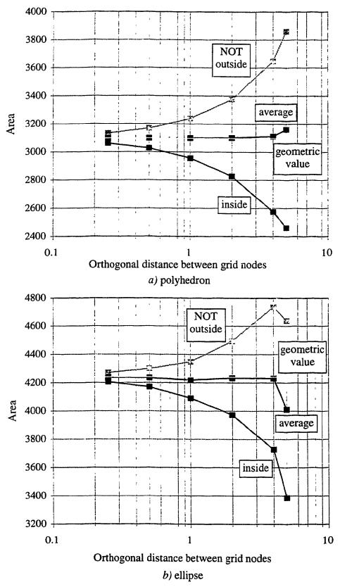
Figure A8.3: Relationship between grid spacing and area calculation
