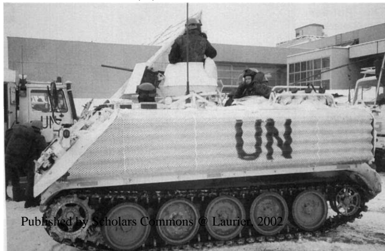
Then (below left): A Danish M113A1 APC in the parking lot of the Sarajevo Airport. This was the standard UN "taxi" for personnel in the city. The armoured shields on the crew commander's hatch and for the pintail mounted .50 cal. M2 Heavy Machine Gun are commonly referred to as Armoured Cavalry (ACAV) Shields as these were first used by the US Army Armoured Cavalry units in Vietnam in the 1960s. Now (below right): The taxis now park a little further down, to the left of the photograph, in order to pick up fares from the newly renovated and repaired terminal. Note that the International Red Cross Volkswagen Golf carries both the red cross and red crescent symbols in recognition of the Christian and Muslim populations in Bosnia.
