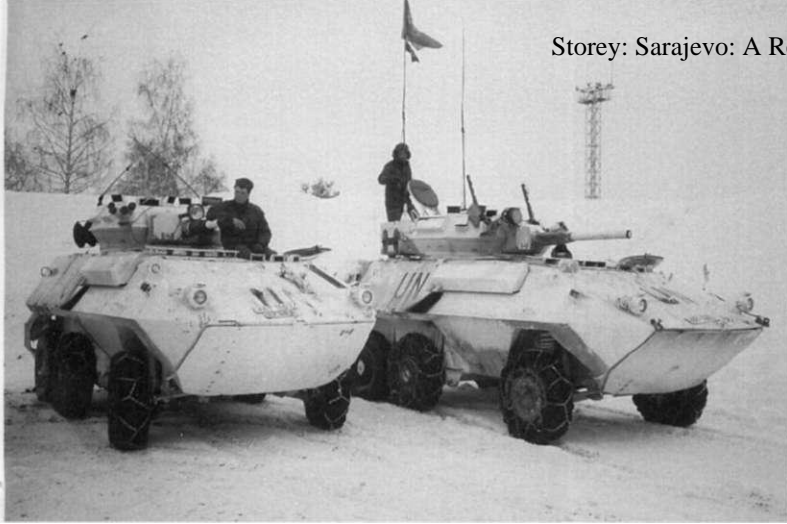
Then (above left): A pair of Canadian Cougar Armoured Vehicle General Purpose (AVGP) at the Sarajevo Airport. Chains are a must on wheeled vehicles, especially those that travel outside of populated regions as the infrastructure to clear and repair the antiquated 1950s-style Bosnian road network had disintegrated during the conflict. Now (above right): The tower with the lights are the base of comparison and the true size of the Airport parking lot is evident in this photograph. Note also the Dobrinja suburb which stretches off into the background as well as the snow on top of Mount Trebevic.
