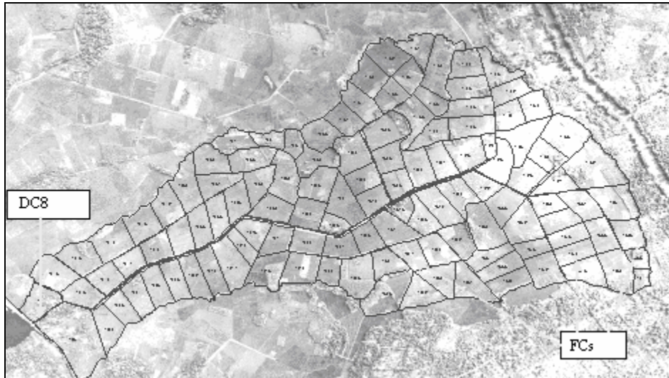
Figure 04: Layout of the Chandrikawewa D8 distributor canal
