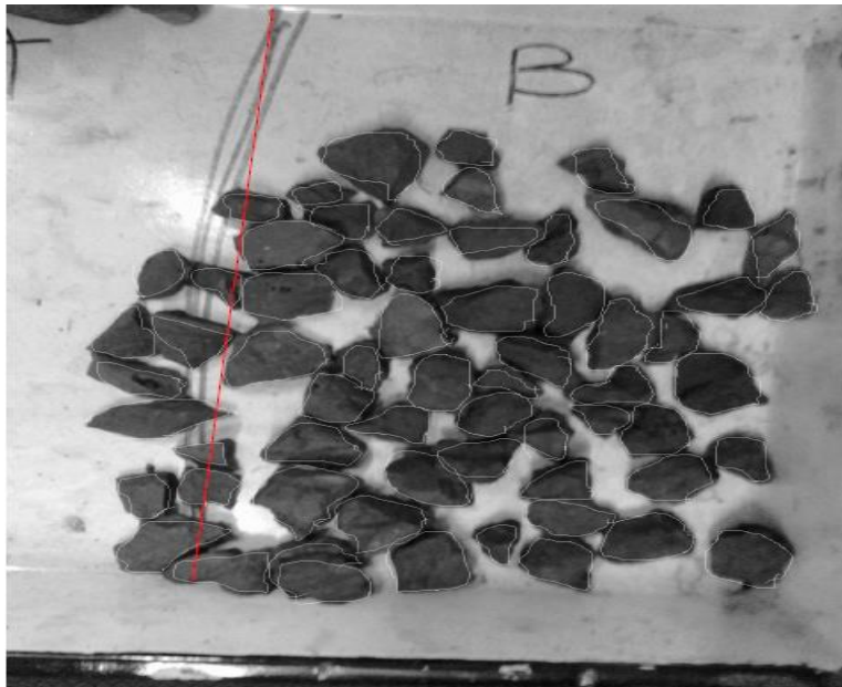
Figure 13: Generated Net of Simple by WipFrag
