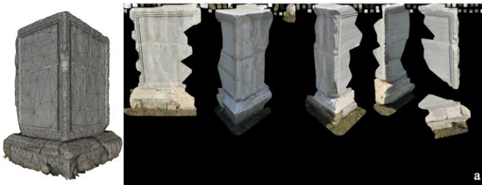
Figure 5. Within a pre-defined LoD, the availability of a large number of photographs determines the accuracy of 3d models, while it doesn't significantly influence the detail of the rebuilt geometry.
