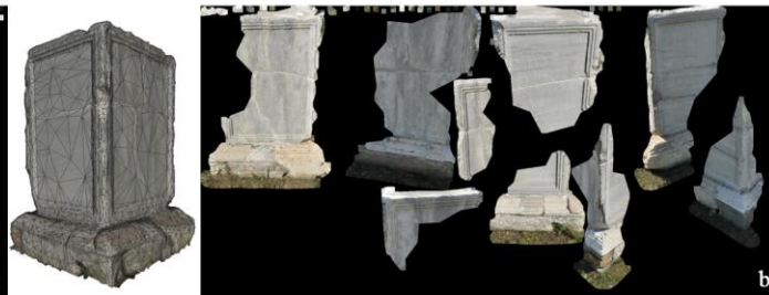
Figure 5. Within a pre-defined LoD, the availability of a large number of photographs determines the accuracy of 3d models, while it doesn't significantly influence the detail of the rebuilt geometry.
