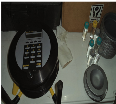
Fig. 4b. Testing of water samples with PHA analyzer (FCI environmental)
