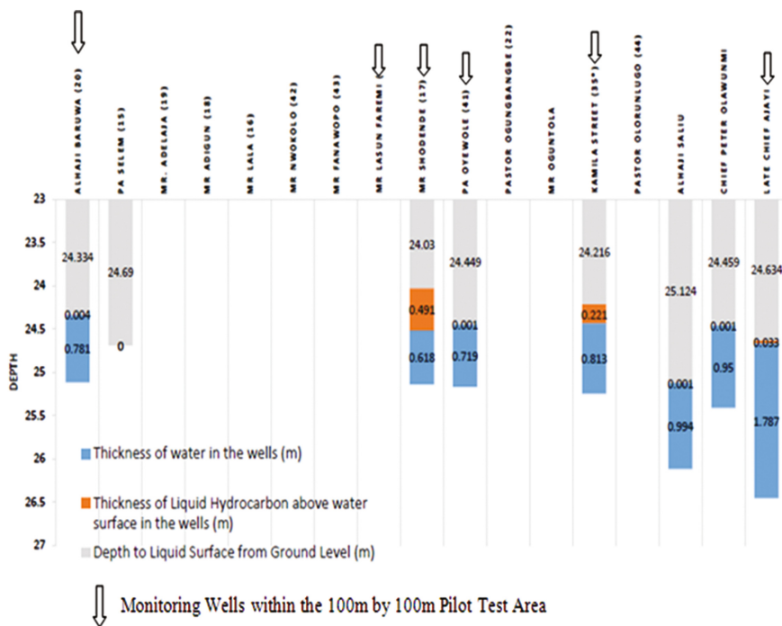
Fig. 5c. Reports of all wells monitored showing the various thicknesses of free hydrocarbon product and water
