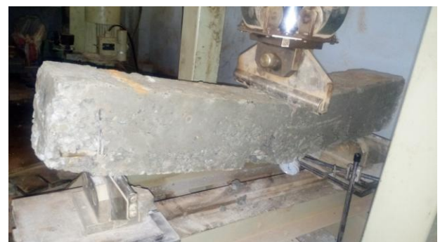
Fig. 10: Failure of beam under applied maximum load
