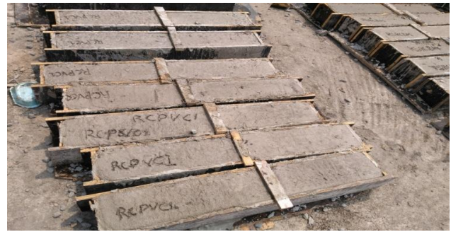
Fig. 7: Casting of beams with and without PVC pipes
