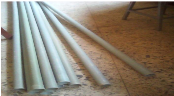
Fig. 5: 50mm diameter PVC pipes
