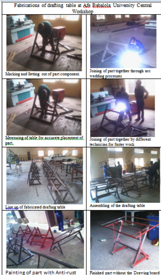
Fig. 10: Fabrication Processes of the drafting Table at the College of Engineering Central workshop, Afe Babalola University, Ado-Ekiti, Nigeria
