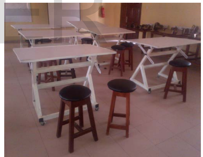
Fig. 12: Photography of Drafting Table Produce at the Design Studio of Mechanical/Mechatronics Department
