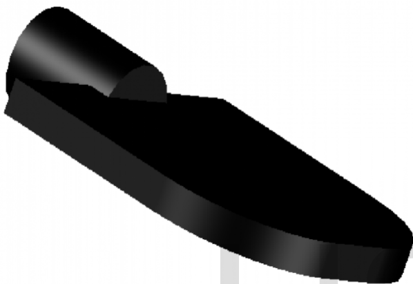
Fig.3: The Screw nod for Angle and Height adjustment
