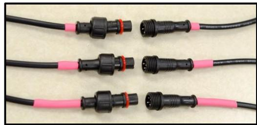
Fig. 22. Color-coded cable joints outside of logger box.
