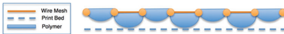
FIG. 3. The heated polymer forms a bulging convex meniscus protruding through the mesh. Here, a dotted line represents the build surface’s substrate that will come in contact with the meniscii during printing, allowing the polymer to wet and adhere to the base material. Color images available online at www.liebertpub.com/3dp
