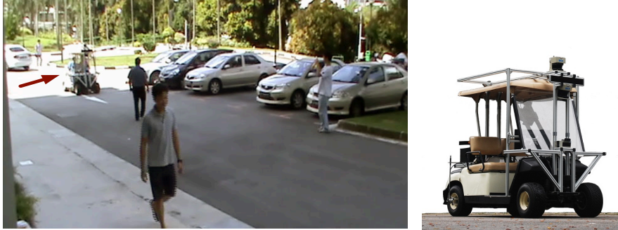
Fig. 1 Our experimental platform, a robot golf cart, during an encounter with pedestrians in a parking lot. Each pedestrian is walking towards one of several goals. Unaware of the pedestrians’ intentions in advance, the vehicle must pass over them as quickly as possible and avoid accidents.
