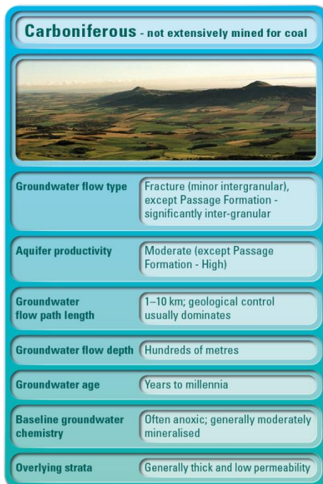
Figure 37 Overview of the hydrogeology of Carboniferous aquifers in Scotland that have not been extensively mined for coal: (top) schematic cross-section; (bottom) summary of aquifer characteristics. From Ó Dochartaigh et al. (2015).
