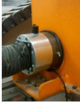
Figure 6-3 AE transducer mounted on the nut
