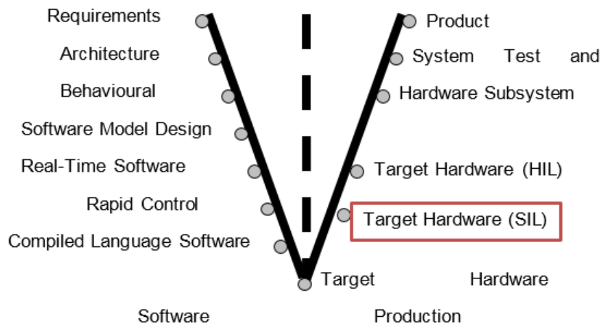
Figure 5-1 V diagram of system engineering
