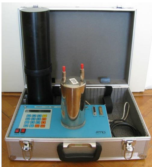
Figure 6: Alpha scintillation cell: a) alpha scintillation cell with PRM-145 alpha scintillation counter, b) schematic view of alpha scintillation cell
