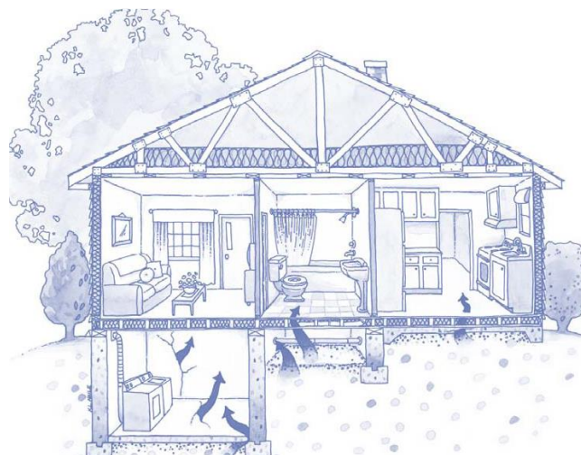
Figure 4: Common radon entry points (U. S. EPA, 2001)
