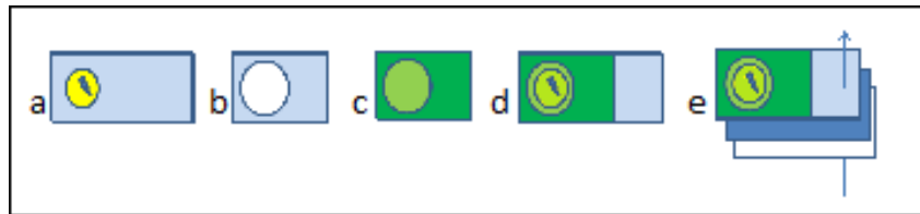
Figure 3.9: Schematic representation of the storage method (light blue = transparent plastic labels; blue = coloured label used for contrast; yellow = glycerol; green = Canada balsam; the pin is represented as a vertical arrow).
