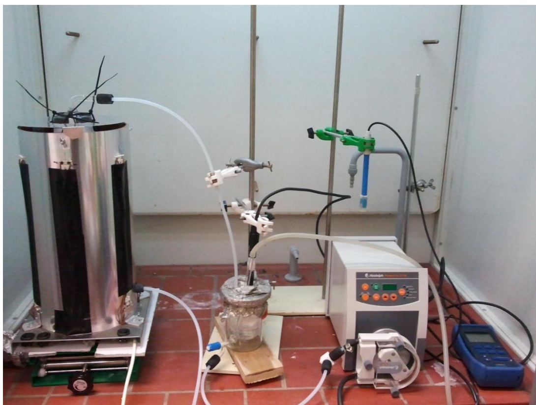
Figure 39. Prototype reactor system with pump and sampling point, where pH, T and O 2 measurements take place (A). Photo of prototype reactor system (B).
