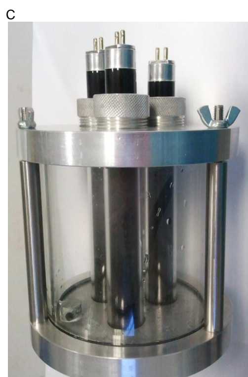
Figure 41. Composition of monolith photocatalytic reactor (A) and photos of foamed ceramic insert (B) and constructed reactor (C).
