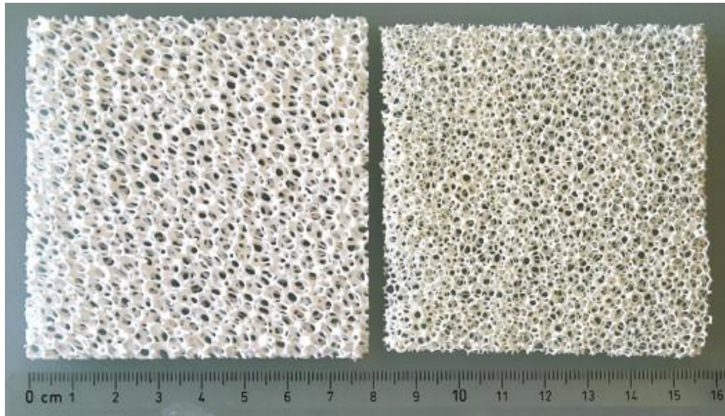
Figure 5. Commercial alumina–mullite Vukopor foam (left) and laboratory made alumina EMPA ceramic foam (right) with the pore dimensions of 15 pores per inch (ppi) (Plesch et al. 2012).
