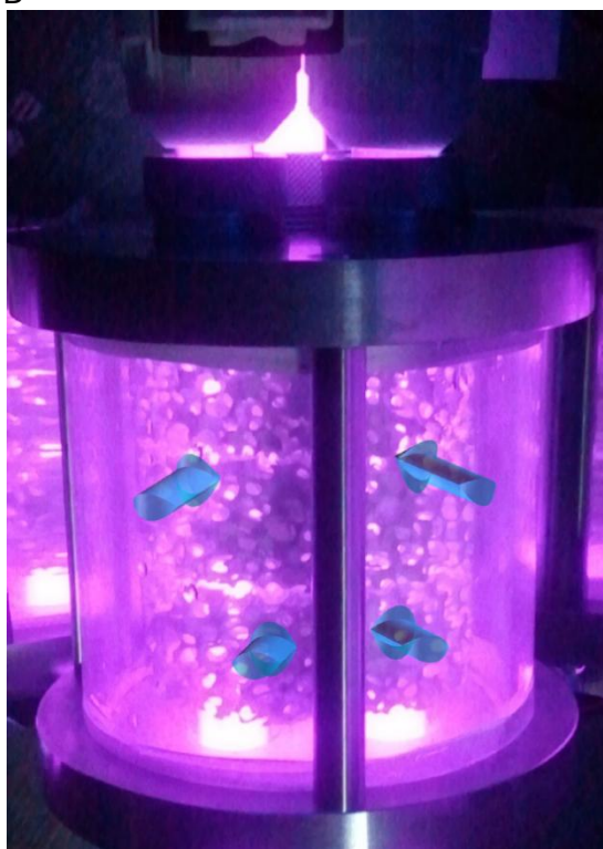
Figure 42. Principle of monolith photocatalytic reactor operation. Tangential inflow forces the water to circle around the monolith (A) and then passes the monolith with immobilized photocatalyst (B).
