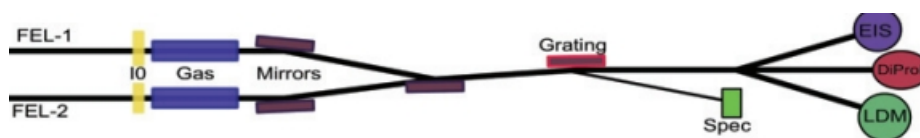
Figure 3.11: Schematic of the FERMI experimental hall including the photon beam transport system and the three experimental chambers. The first part of the FEL front hand includes, for both FEL1 and FEL2, two ionization chamber intensity monitors and a gas cell providing a wide range tunable intensity attenuation. Then, the light impinges on a variable spacing grating positioned to direct the first diffraction order, 3% of radiation power, onto a YAG screen with fluorescent intensity detected by a CCD while the zeroth order goes to one of the experimental stations. This system permits to measure the FEL spectrum during user operation. Courtesy of D. Cocco.
