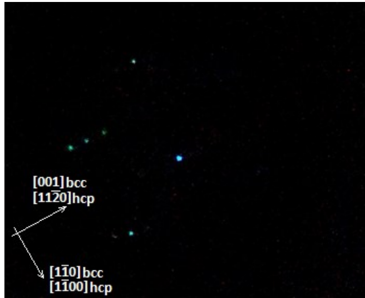
Fig. 4.2 LEED pattern after 4 min of total Co deposition. Arrows indicate [001]_{\text{bcc}} of Mo and [11-20]_{\text{hcp}} of Co in one direction and [1-10]_{\text{bcc}} of Mo and [1-100]_{\text{hcp}} of Co in other direction. E=143.5\text{eV}
