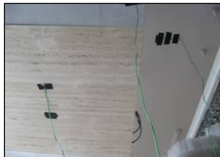
Fig 23: Thermocouples on panels and ceiling
