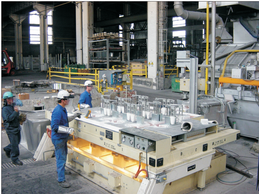
Figure 1.2: A DC billet casting machine in the Impol casthouse. Photo by Božidar Šarler.
