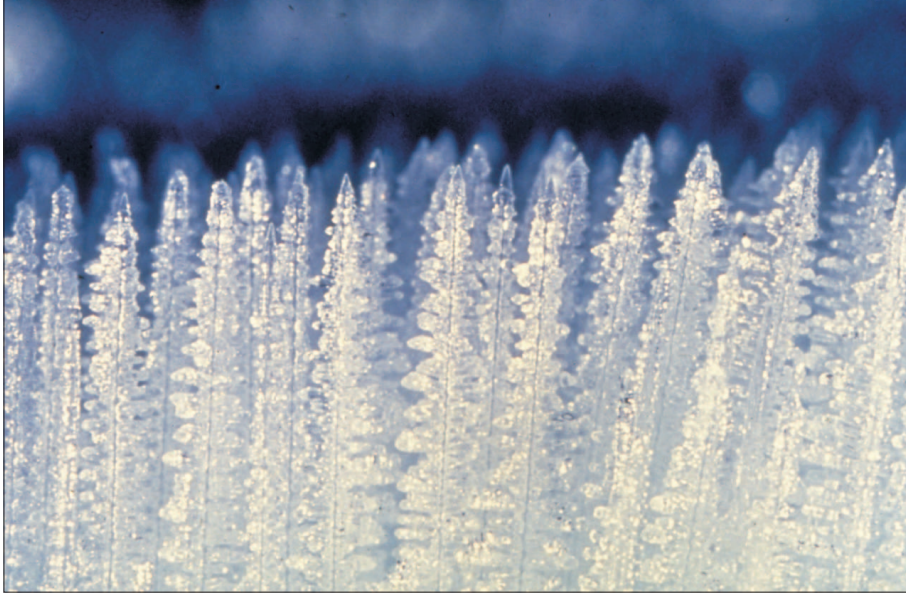
Figure 1.6: Columnar mushy zone in a solidifying ammonium chloride solution [Huppert and Worster, 1985]. Photo by Mark Hallworth, courtesy of M. Grae Worster, University of Cambridge.
