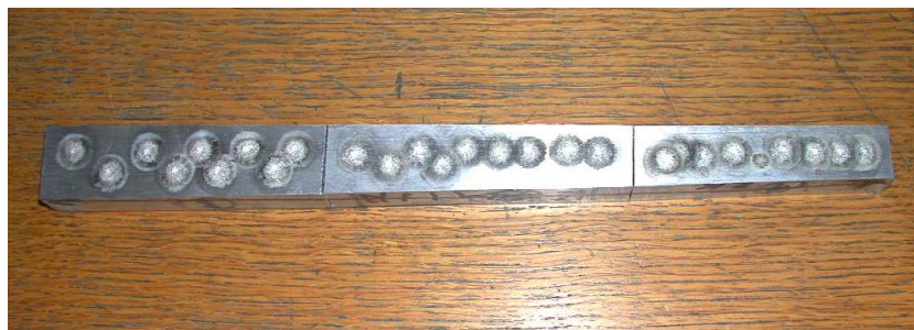
Figure C.1: Optical emission spectrometry sample of the first billet section (Profile 1 in Fig. C.2).
