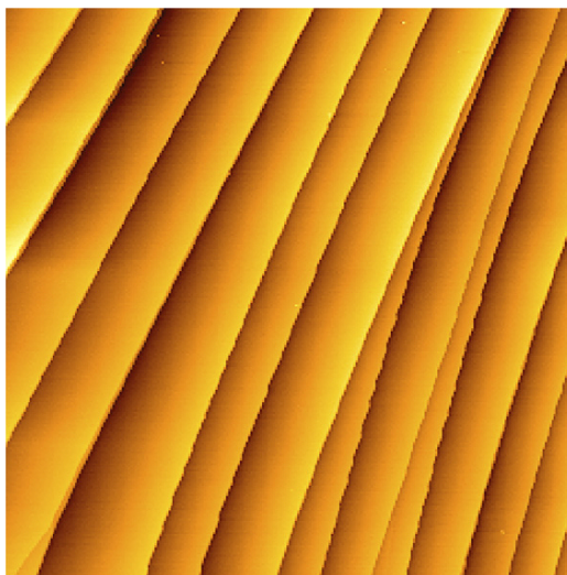
Figure 5.1: A 4 \times 4 \mu\text{m}^2 AFM image of a sapphire substrate annealed at 1500^\circ\text{C} for 120 h. The surface is characterized by terraces separated by steps which on average measure 2.8 nm in height.
