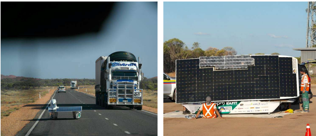
Figure 4.3: Primavera 2 Solar Vehicle Cruising in Stuart Highway and charging process during 30 minute mandatory control-stop
