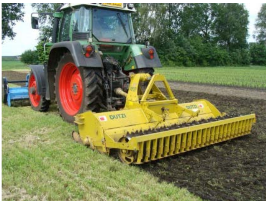
Figure 49 The incorporation of a grass-clover sod with a hooks cutter ( www.wageningenur.nl )
