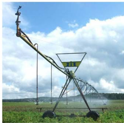
Figure 82: Schemata of a centre pivot irrigation system (blue = irrigated, green = unirrigated); picture of a centre pivot system with swing arm at the end (source: Mersch & von Haaren)
