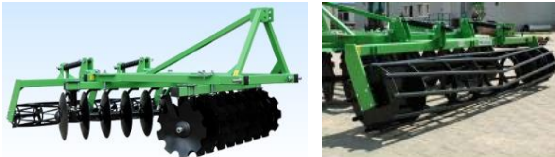
Figure 34: Disc harrow with 2 rollers; tubular roller ( http://www.bomet.pl )
