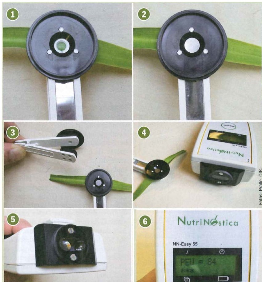
Figure 68: Application of manganese sensor (Olf & Pralle 2010)
