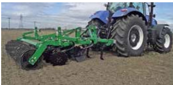
Figure 43: Examples of different vertical tillage equipment ( http://www.greatplainsag.com/ )
