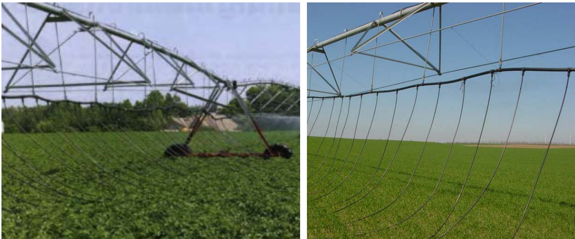
Figure 81: Mobile drip irrigation (drip tubes) with center pivot irrigation machines for potatoes (source: Lüttger); mobile drip irrigation (drip tubes) with center pivot irrigation machine (source: Sourell et al. 2014)
