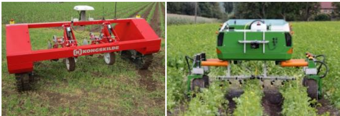
Figure 76: New automated agricultural platform ( www.kongskilde.com ); Multi-functional field robot for agricultural applications ( www.amazone.de )
