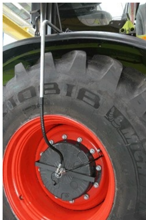
Figure 92: Low pressure tires with remote control of pressure ( www.michelin-pneu-agricole.fr )
