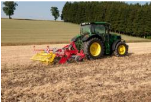
Figure 28: Compact disc harrow ( http://www.poettinger.at/landtechnik/download/237.02.0113_Terradisc_en.pdf )
