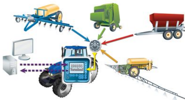
Figure 53: ISOBUS Terminal to implement machines from different manufactures and to exchange data between PC and terminal ( http://www.teejet.de/german/home/products/application-control-and-equipment/isobus-and-iso-11783-solutions/about-isobus.aspx )
