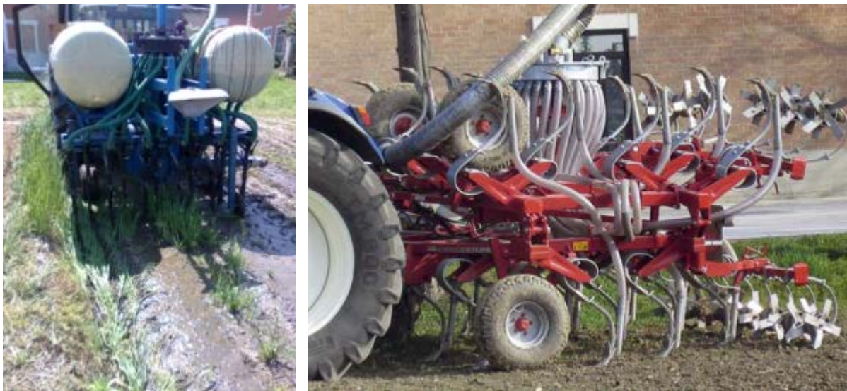
Figure 71: Trailing shoe distribution system or slurry injection device (source: Riva et al. 2013)
