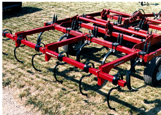
Figure 26: Chisel plow ( http://www.deere.com/common/media/images/product/tillage/primary_tillage/610_integral_chisel_plow/610_IntegralChiselPlow_0027064_642x462.png ; http://www.farmequipmentfinder.com/view_item.php?id=2646 )
