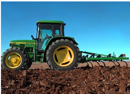
Figure 26: Chisel plow ( http://www.deere.com/common/media/images/product/tillage/primary_tillage/610_integral_chisel_plow/610_IntegralChiselPlow_0027064_642x462.png ; http://www.farmequipmentfinder.com/view_item.php?id=2646 )
