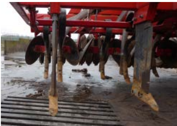
Figure 72: The manure injectors are positioned at each side of the to be planted maize row (left); two manure rows at 12 cm deep are placed and registered with DGPS. In a day, the maize seed is planted exactly in between the manure rows (right; http://edepot.wur.nl/206790 )
