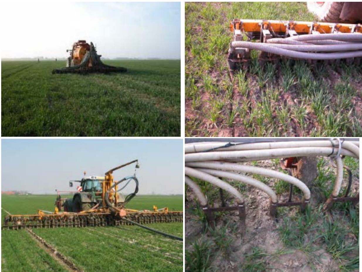
Figure 65: Tractor with tank and slurry injector (top left), detail of slurry injector (top right) and drag hose supply with slot coulters (bottom left) and detail of slot coulters (bottom right) (source: Huijsmans et al. 2012; http://edepot.wur.nl/203220 )
