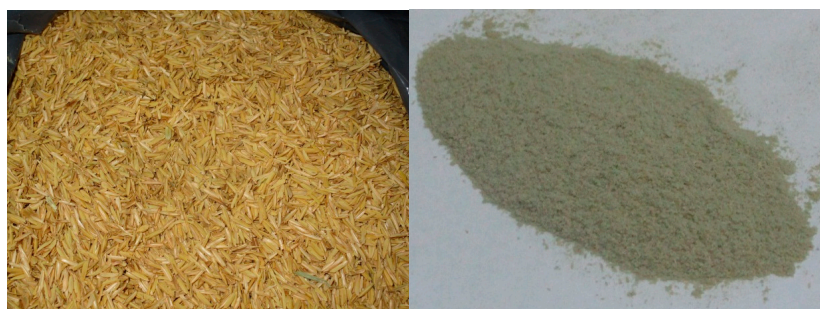
Figure 5. Pretreatment of rice husk (left image) to fine sieved powder (right image) via milling prior to processing.
