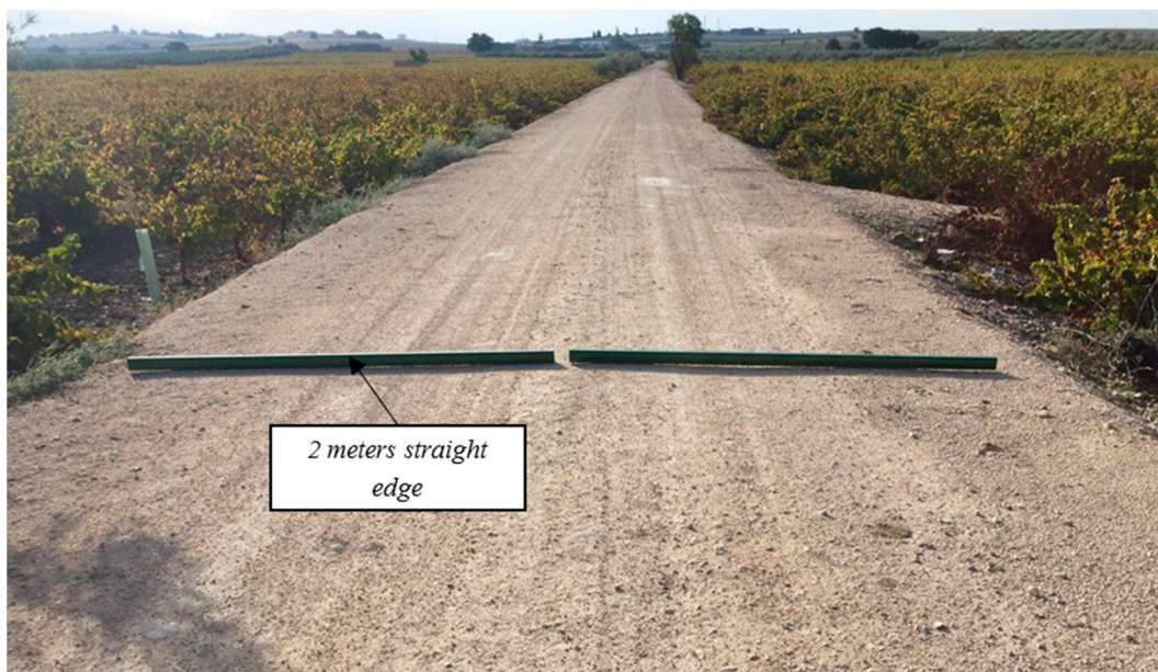
Figure 5. Straight edge of 2 m in each wheel path.
