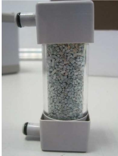
*Figura 39. Detalle Soda Lime.*
