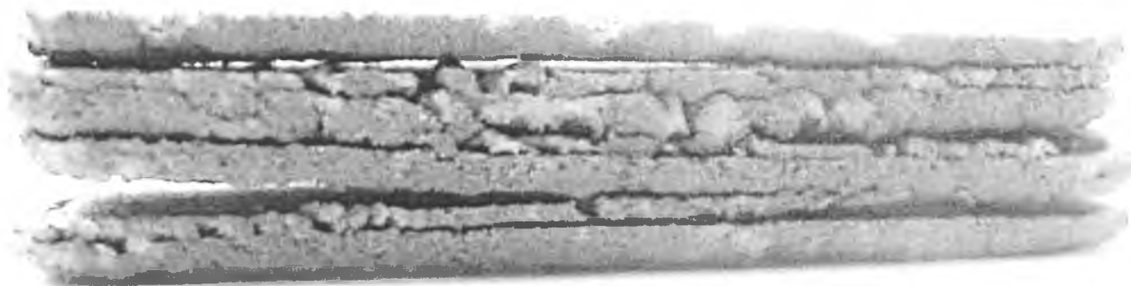
Figure 7.30: Eight Layer with different scan direction using layer thickness 1.0 mm, laser power = 75W, scan speed = 1mm/s, and scan spacing = 0.682mm
