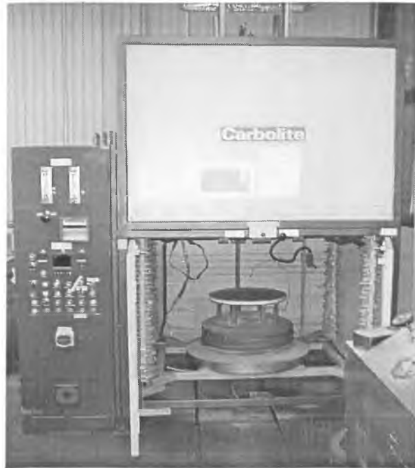
Figure 4.2: Carbolite Furnace for RapidSteel 2.0 post-processing
