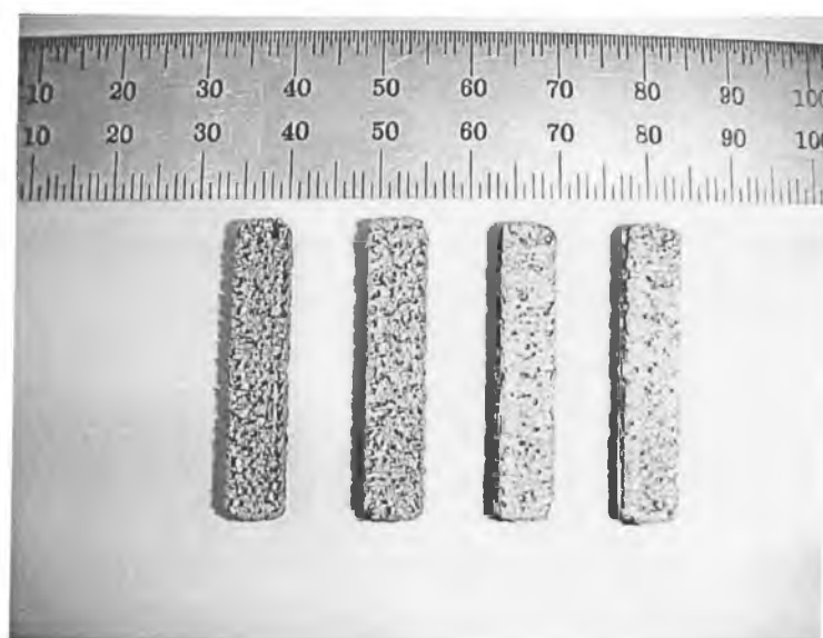
Figure 7.34: Four samples with layer thickness 0.6 mm each
