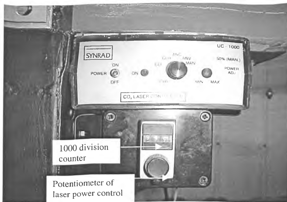
Figure 6.8: Photograph showing the UC-1000 laser controller with the additional potentiometer and numerical counter
