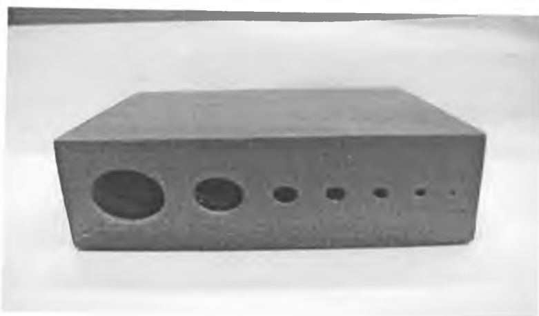
Figure 5.41: Brown part with different diameter channels.
