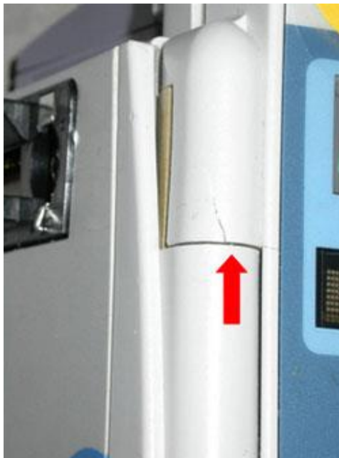
Figure 2-11: Image showing a cracked door hinge resulting from stress caused by misaligned tube [23]
