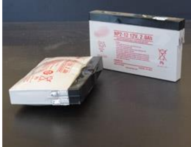
Figure 2-12: Image showing sealed lead-acid battery damage [23]
