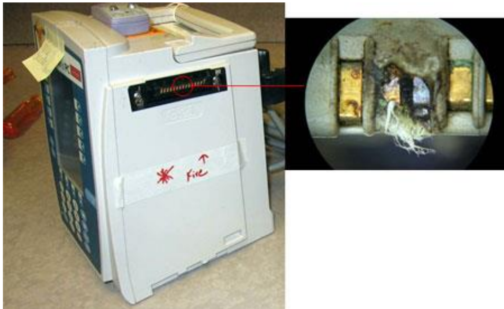
Figure 2-13: Image showing the charring and melting of failed connectors [23]
