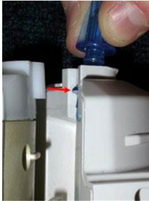
Figure 2-10: Close up image of the tubing set out of alignment [23]
