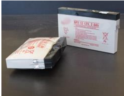
Figure 8-11: Image showing sealed lead-acid battery damage [23]
