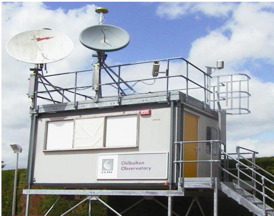
Figure 3.3 The hut at Sparsholt where the receiving antennas have been installed along with the data logging system [46].
