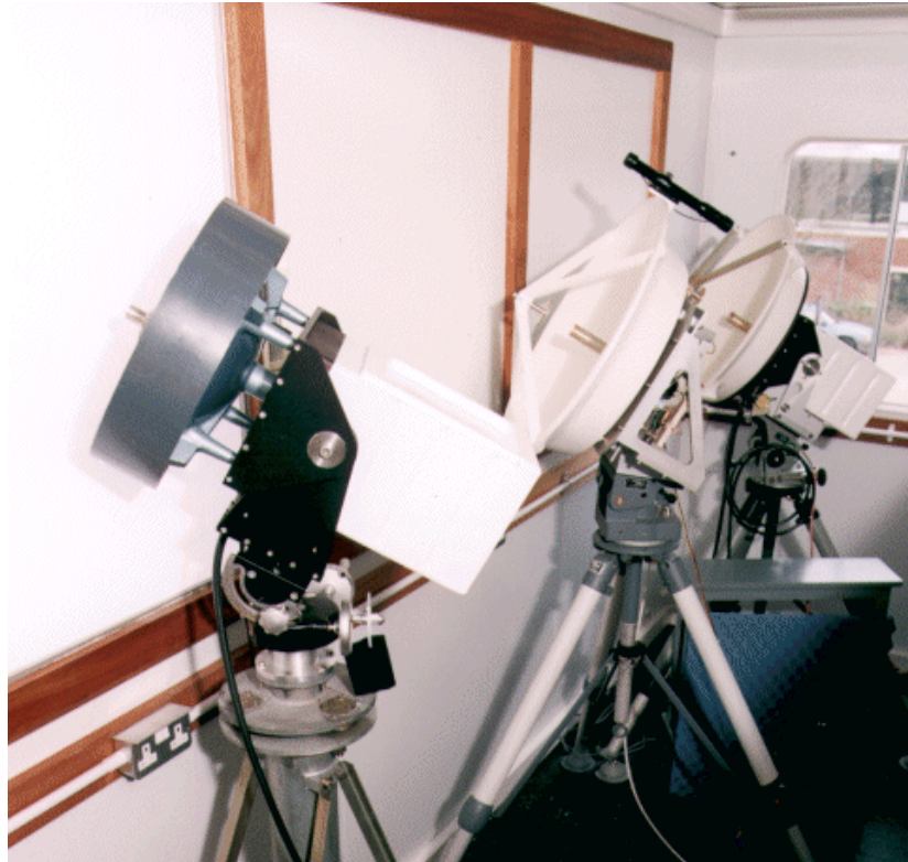
Figure 3.4 From left to right, the 51GHz radiometer, the 50GHz receiver and the 40GHz receiver [46].
