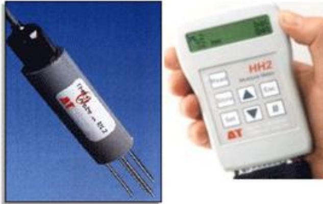
Figure 3-5: Shows the Theta Probe ML2X for the measurement of the moisture sensor
