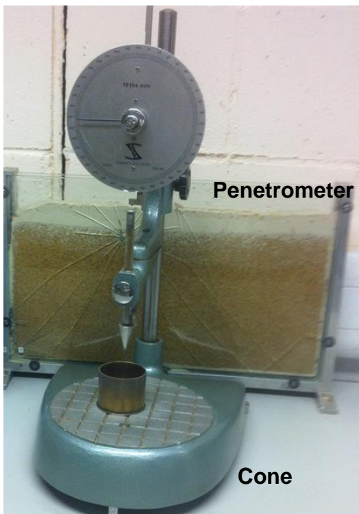
Figure 3-7: Shows the penetrometer and cone used to determine the liquid limit
