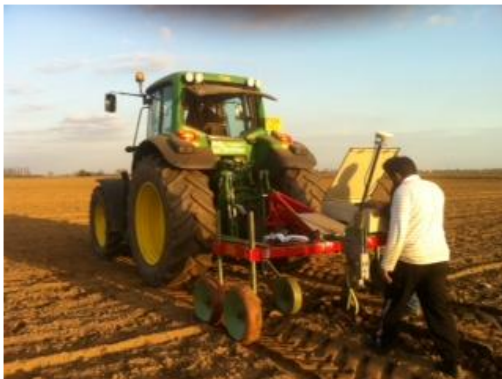
Figure 3-3 : Illustrates the multi-sensor platform for on-line measurement of soil properties (Mouazen, 2006)
