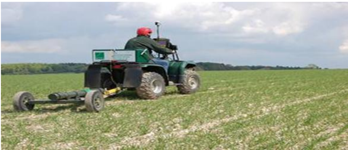
Figure 3-4: Shows the Dualem 1S sensor with a quad bike during field measurement
