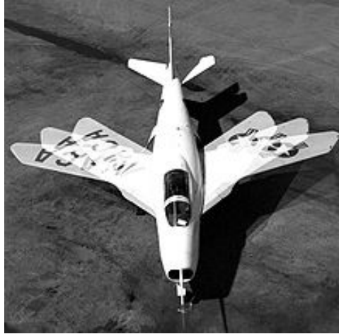
Figure 2.15: Bell X-5 variable sweep wing [22]
