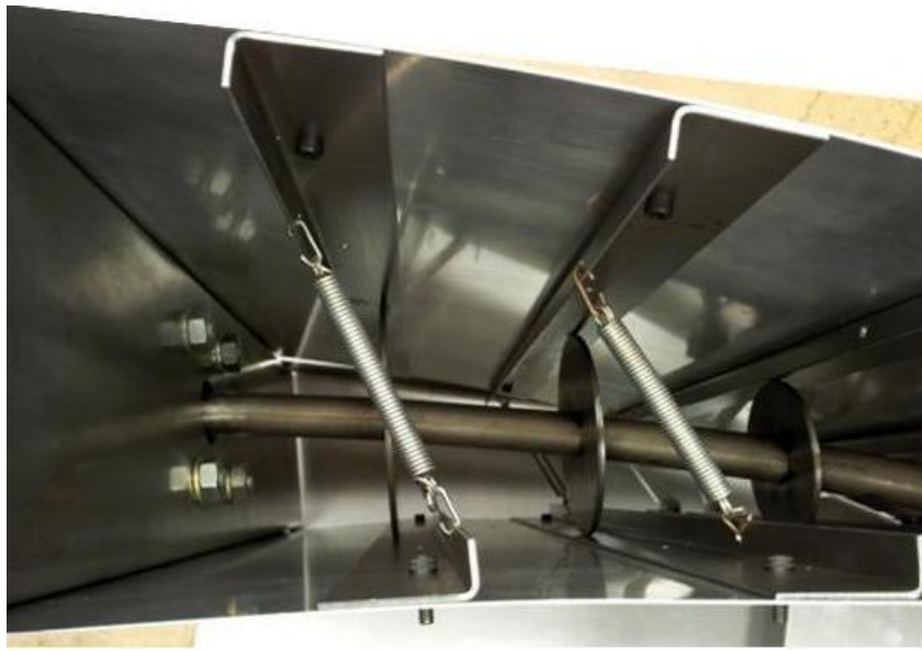
Figure 5.17: Internal structure of the flap
