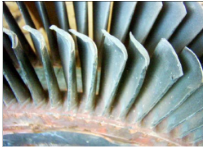
Figure 7-1 Creep attack Impact on Turbine Blades [77]
