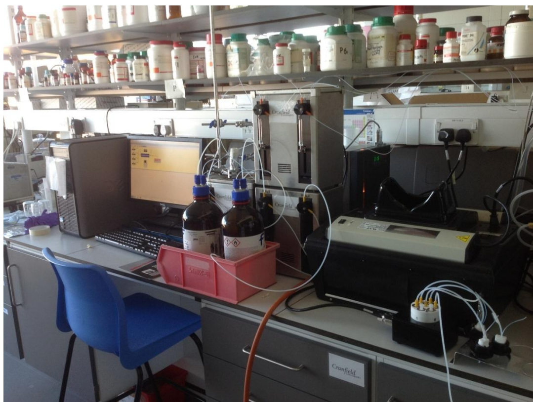
Figure 3–20. Picture of the automated solid-phase MIP NPs photoreactor.
