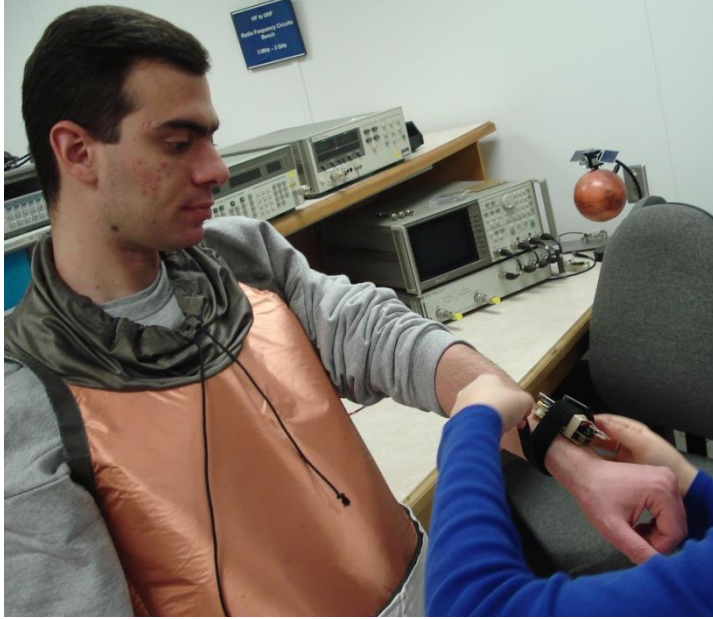
Figure 3.16 Placing Antenna on the Arm
