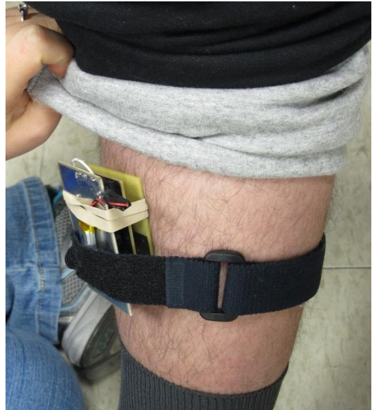
Figure 3.20 Close up of Antenna, Radio, and Audio Oscillator on Leg
