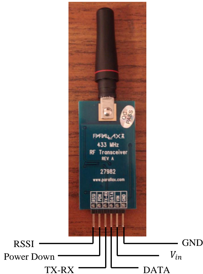
Figure 3.8 Radio Inputs and Outputs Interface
