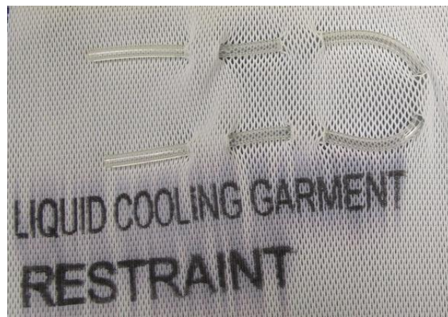
Figure 4.2 Liquid Cooling Garment in Sample From ILC Dover used in Current Suits
