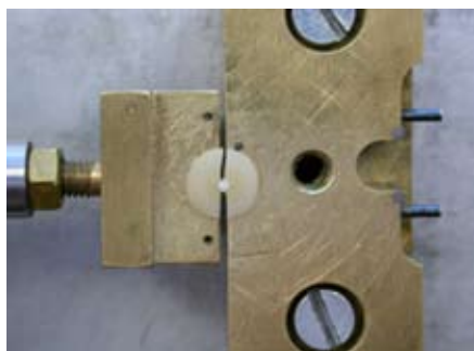
Fig. 2. A specimen attached to the SMAC actuator for testing.
