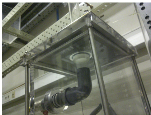
Figure 2.15: Pre-chamber in the first tested configuration.
