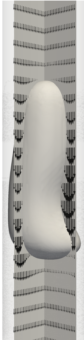
Figure 4.3: Drop and velocity field (drop nose reference frame) for Eo = 22 , M = 100 and \mu^* = 10 .
