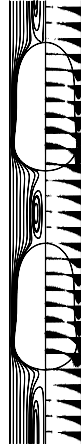
Figure 6.7: Velocity field and streamlines (leadind drop reference frame) for M = 100 , Eo = 8 , \mu^* = 10 and u^* = 2 .
