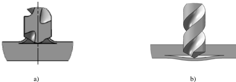
Figure 1 Delamination mechanisms: a) Peel-up; b) Push-down.
