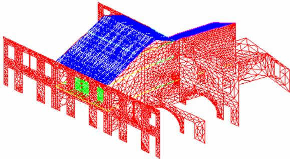
Fig. 13 – House no. 15. New numerical model.
