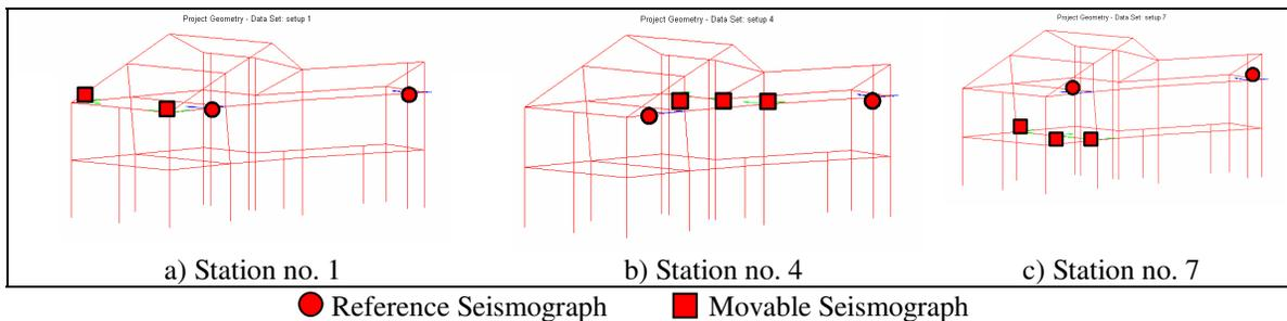
Fig. 15 – House no. 15. Some ambient vibration measuring stations
