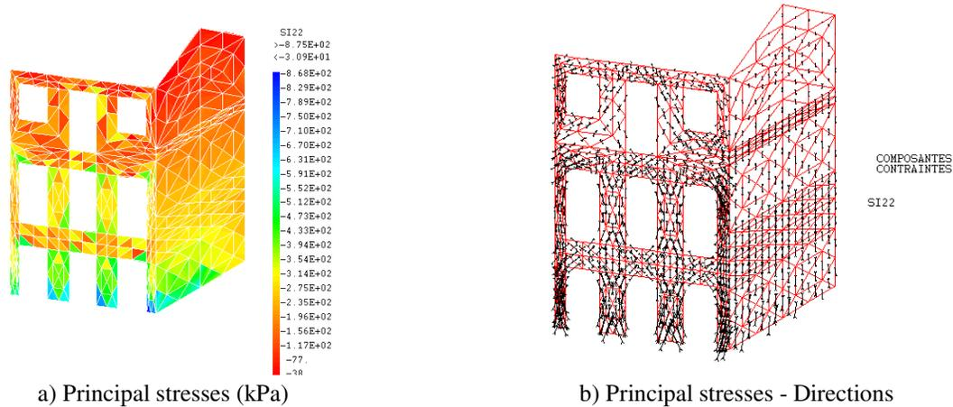
Fig. 26 – House 16 - Principal Stresses (Compression) due to seismic loads – Frontal Wall
