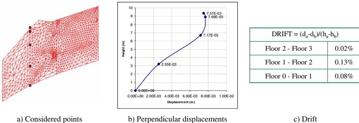
Fig. 27 - House no 15 - lateral wall – displacements
