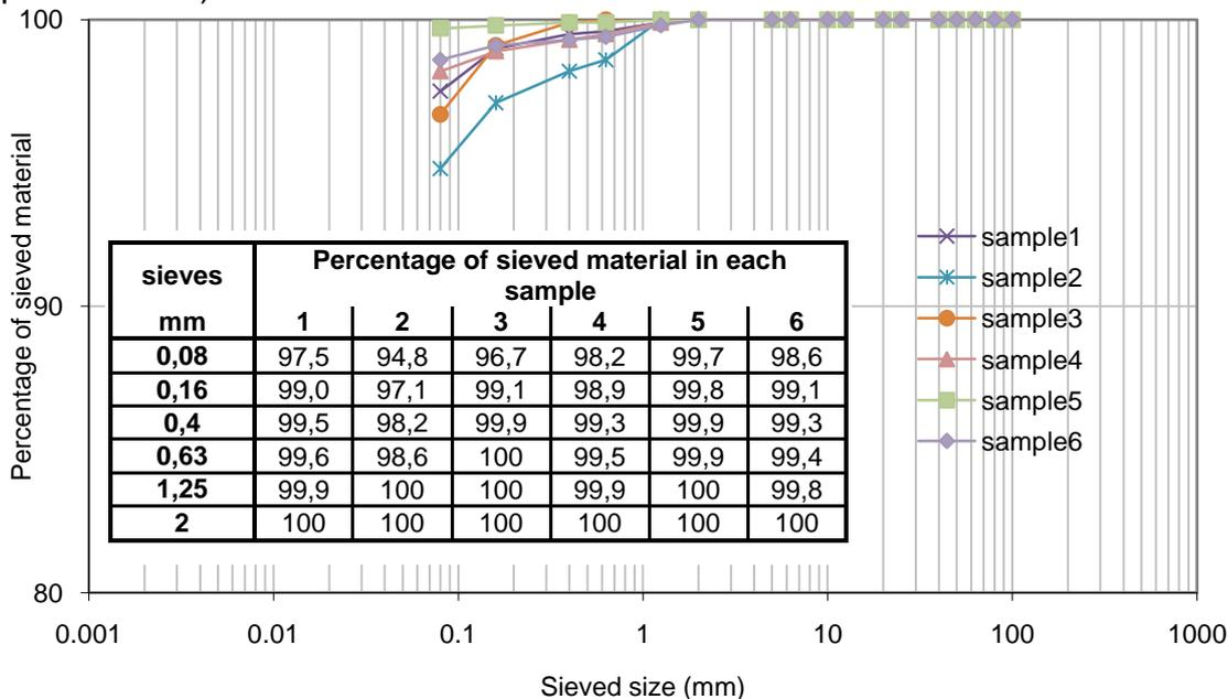
Figure 4 – Grading curves of natural soil samples.
