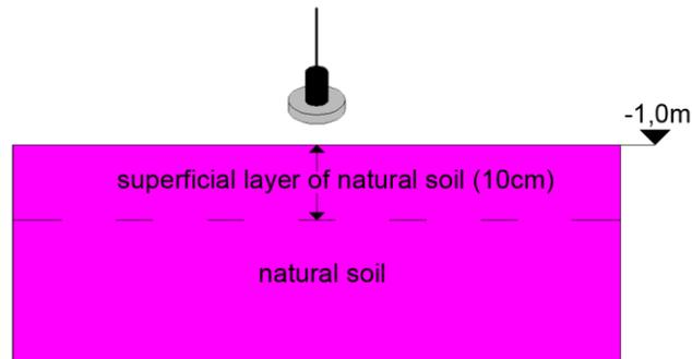
Figure 8 – Structure of the pavement foundation - areas 1 and 2
