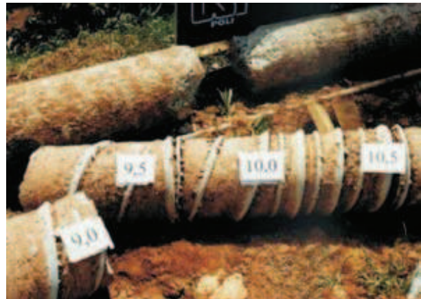
Figure 29 - Omega pile in 9.0 to 10.5 m depth segment.
