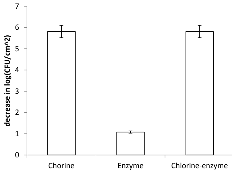
Figure 5 – Adhesion of microorganisms to stainless steel 316 after treatment with the different strategies with agitation of 150 rpm. *means 0 CFU (a). Decrease in adhesion of microorganisms to stainless steel 316 after treatment with the different strategies with agitation of 150 rpm (b). The mean \pm standard deviation of, at least, three replicates is illustrated.
