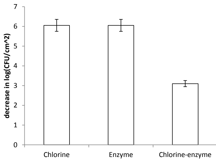
Figure 7 – E. coli adhered on HDPE after treatment with the different strategies with agitation of 150 rpm. *means CFU (a) . Decrease in adhesion of microorganisms to HDPE after treatment with the different strategies with agitation of 150 rpm (b) . The mean \pm standard deviation of, at least, three replicates is illustrated.
