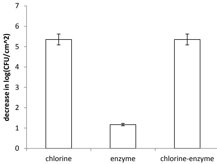
Figure 4 – Adhesion of microorganisms to stainless steel 316 after treatment with the different strategies under static conditions. * means 0 CFU (a). Decrease in adhesion of microorganisms to stainless steel 316 after treatment with the different strategies under static conditions (b). The mean \pm standard deviation of, at least, three replicates is illustrated.
