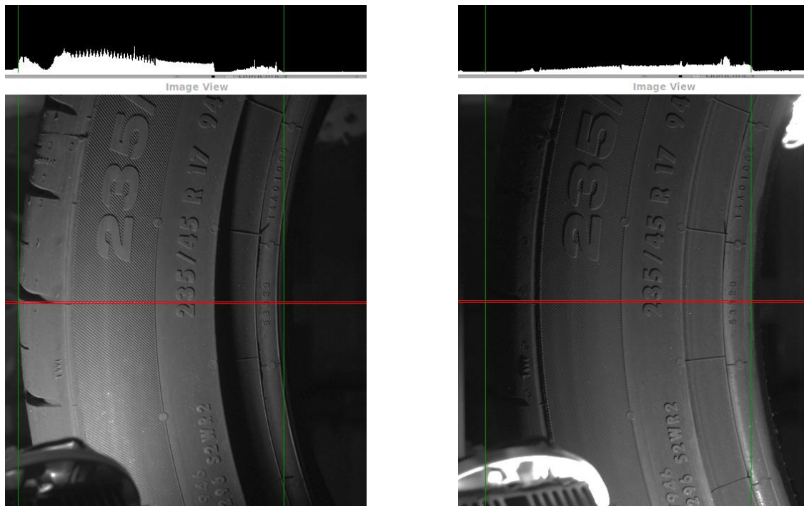
Figure 4.18 - Example of user interface environment when defining a lighting configuration. The window being captured is shown in red. On top of each image the intensity profile is plotted. In the left image only the bottom LED array is emitting light and on the right, only the top LED array is on.
