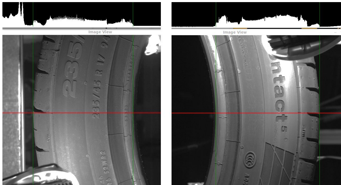
Figure 4.19 - Lighting configuration for a conforming tire. On left the inside sidewall and on the right the outside sidewall of the same tire are shown.
