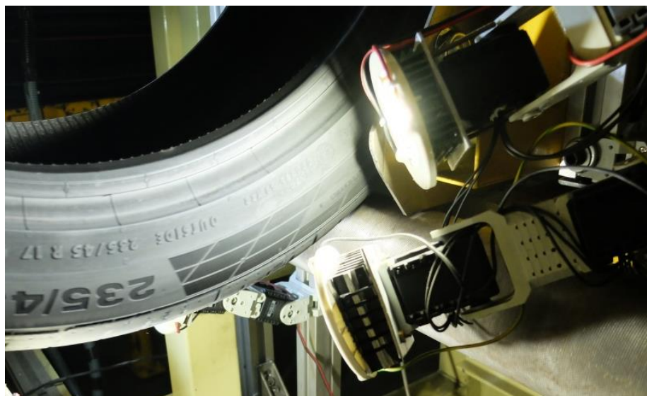
Figure 4.17 - Pictures of the prototype: in the top image the articulated arms are in the home position, while in the bottom image an acquisition is taking place.
