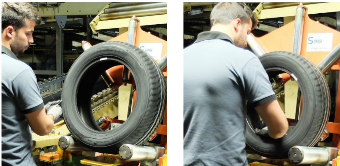
Figure 2.12 - Visual and Haptic Search in the tire quality inspection process. On the left a detail of a simultaneous downward sidewall observation and trimming is shown while on the right the operator is inspecting the inner liner both visually and haptically.
