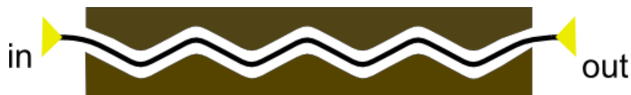
Figure 29: Schematic drawing of a microbending sensor.
