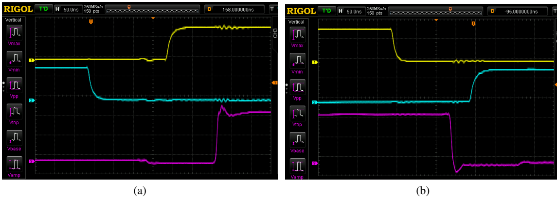
Figure A.2: Oscilloscope print of the difference between defined and real dead time for both edges. The two signals are measured at the output pins of the microcontroller while the bottom one is measured at the swithing node voltage.
