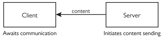
Figure 5.10: Push model diagram
