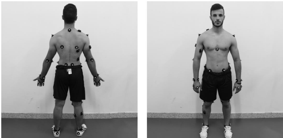
Figure 4.7. A sample map for EMG sensors and reflective markers placements.
