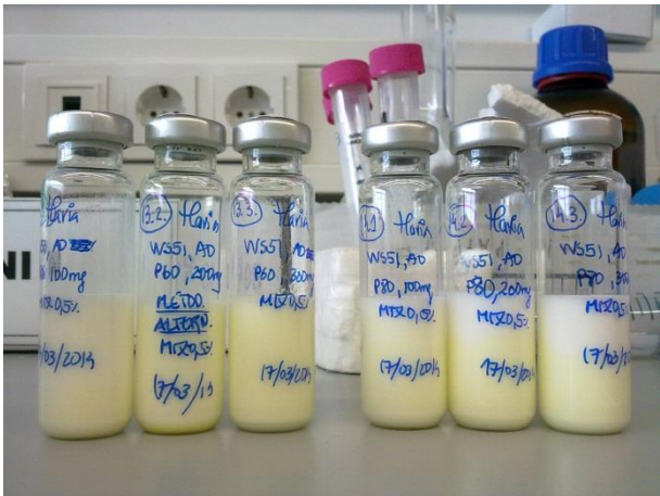
Figure A5. Aspect of the NLCs formulations D.1.2.7., D.1.2-ALT and D.1.2.8. with polysorbate 60 as the surfactant, and D.1.2.9.-D.1.2.11. with polysorbate 80.
