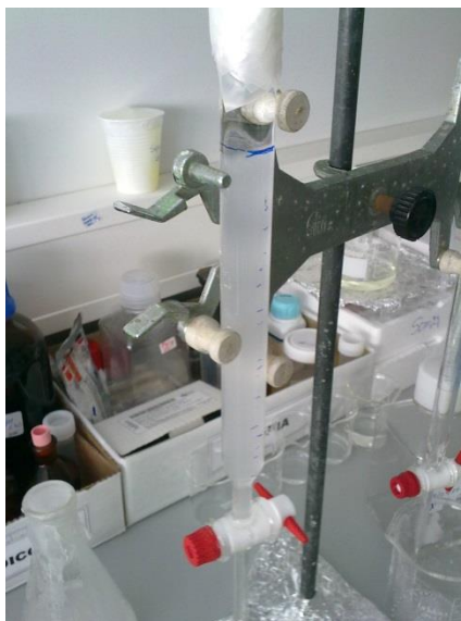
Figure A1. Sephadex column utilized for the separation of NLCs from unincorporated drug by gel filtration.
