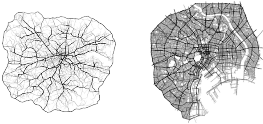
Fig. 17 – The dual structure of urban street networks as revealed by configurational analysis. Dark lines are more central, light grey lines more segregated. The images show the pattern of global choice (a type of centrality) for London (left) and for Tokyo (right). Source: (Hillier 2009).
