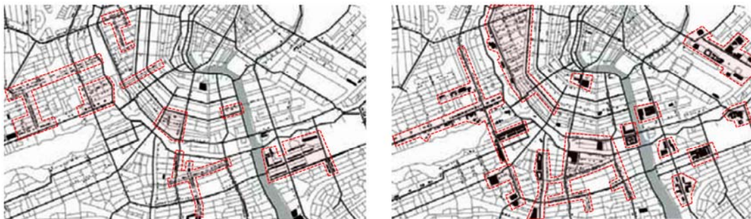
Fig. 20 – The coincidence between movement grid and urban functions. On the left: local-scaled grid and local functions; on the right: middle-scaled grid and city-scale functions. On both images the local-scaled grid is light and the middle-scaled grid is dark. Source: (Read and Bruyns 2007)
