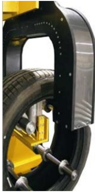
Figure 2.10: YXLON bead spread technology ( source: YXLON [5] )
