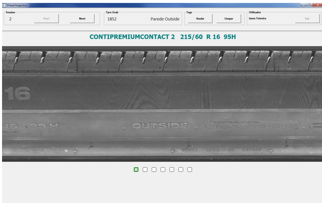
Figure 5.14: Virtual Inspection interface: enhanced version
