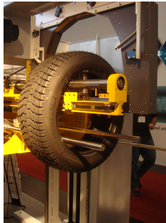
Figure 4.3: X-ray test machine handling solution
