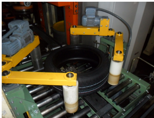
Figure 2.2: Bead Lubricant Applicant (Uniformity Machine) handling solution
