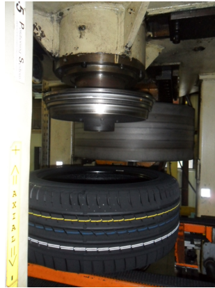
Figure 2.3: Uniformity Machine Test Area handling solution
