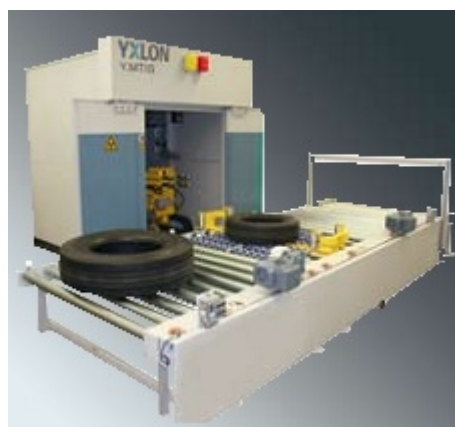
Figure 2.9: Y.MTIS Family TBR solution from YXLON ( source: YXLON [5] )
