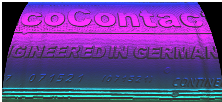
Figure 4.31: 3D image gathered from tire sidewall
