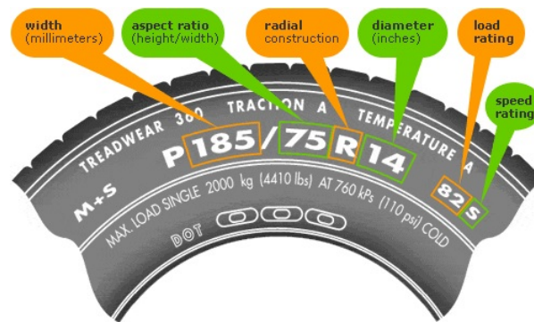
Figure 1.4: Meaning of the different tire dimensions placed in the tire sidewall ( source: Engine Basics [3])
