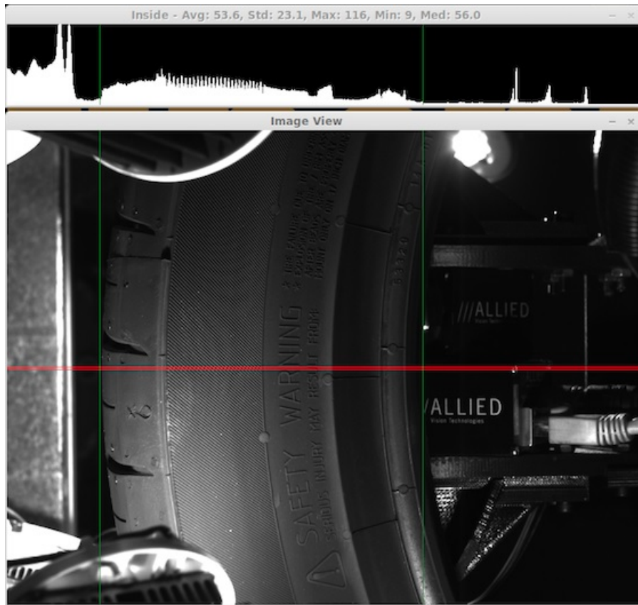
Figure 3.8: Tool available in the tire grabber applications to support the lighting setup
