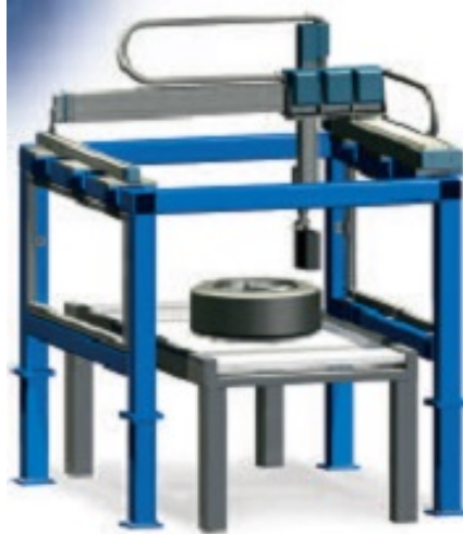
Figure 2.7: DOT read-out application handling solutions
