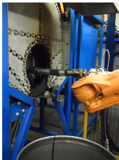
Figure 2.5: ContiSeal Sealant Application handling solution
