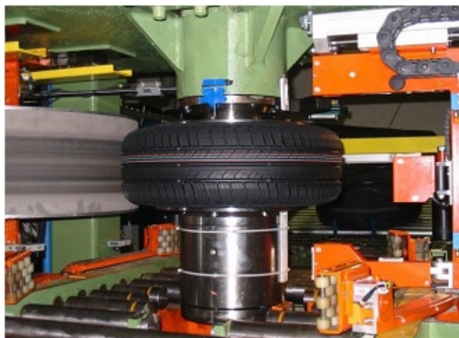
Figure 2.12: Tire Surface Inspection solution from Micro-Epsilon
