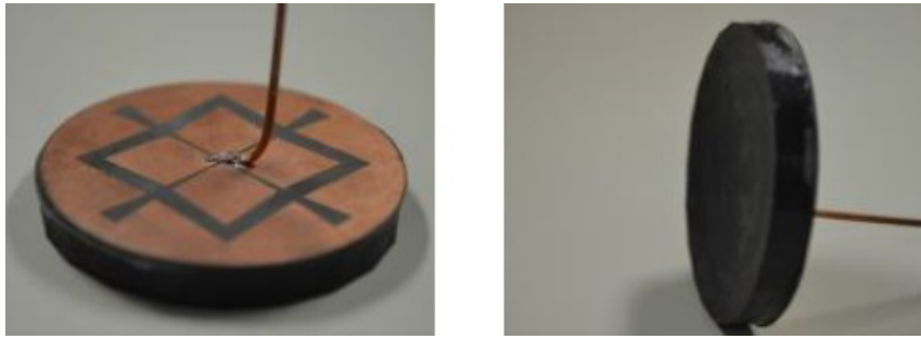
Figure 2.4: Representation of the conformal antenna used [4].
