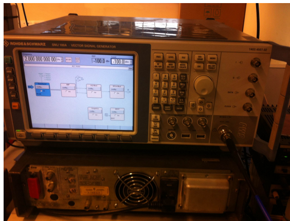
Figure 3.10: Power source used in the experimental setup of the phantom heating.
